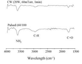
FIJI FT-IR of continuous wave (at 20 W, 60 mTorr and 1 min) and pulsed (60/100) plasma polymerization coatings.
